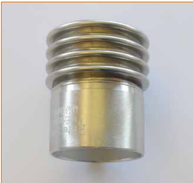
Circumferential welding | hand-held torch (3.0 mm on 0.2 mm)
