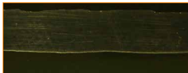
Repair welding with DualWave. Far fewer pores.
