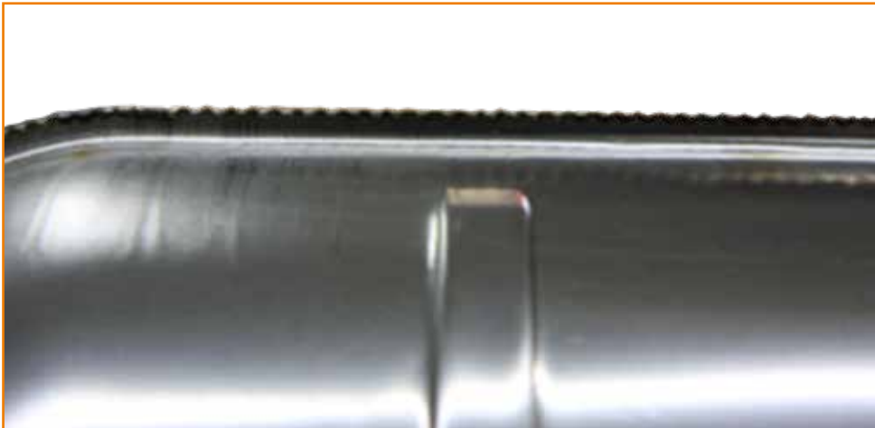
Stainless steel tank with 250 tack welds
